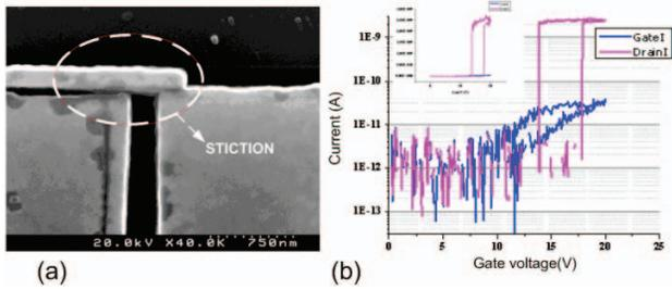
Fig. 2. (a) SEM image showing stiction in a SiC cantilever beam; b) the log plot shows switching characteristics of a typical SiC 3-terminal device with  $8\mu\text{m}$  length beam and  $250\text{nm}$  gate-source gap (inset: linear plot).
