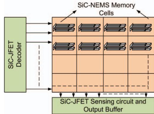
Fig. 3. Block diagram showing JFET-NEMS integration to realize memory array: JFET peripheral electronics and NEMS 5T memory cells.
