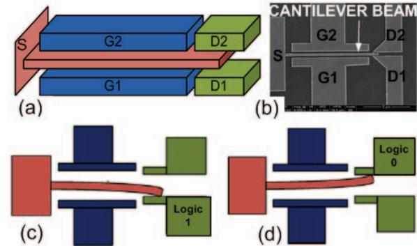
Fig. 1. (a) Schematic of the proposed 5T nanomechanical memory cell; b) an SEM image of the 5T device; c) and d) bi-stable nature of the cells representing stored content of '1' and '0', respectively.
