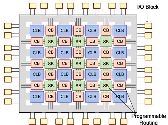
Figure 2. FPGA architecture consisting of interlaced configurable logic blocks (CLBs) and programmable interconnect (CB: Connection Box; SB: Switch Box).
