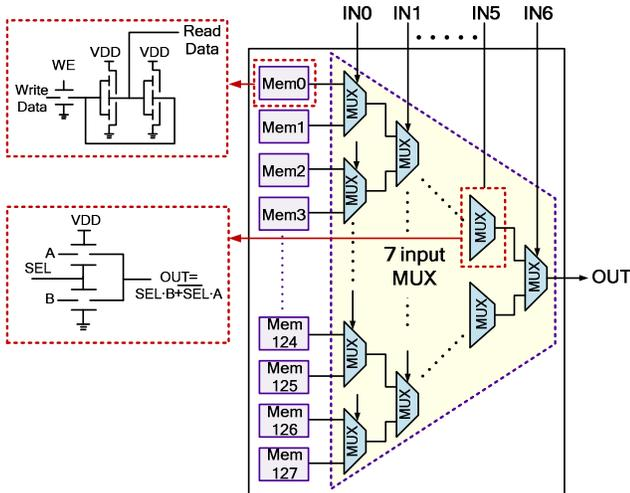
Figure 5. 7-input LUT with NEMS switch level schematic of the memory elements and the MUX tree.
