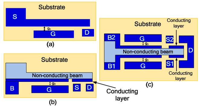
Figure 4. (a) 3-T NEMS single-layer switch; (b) 4-T NEMS multi-layer switch; (c) 7-T NEMS multi-layer switch for efficient implementation of 2x1 multiplexer.
