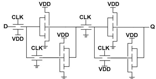
Figure 6. NEMS switch level schematic of a D flip-flop.
