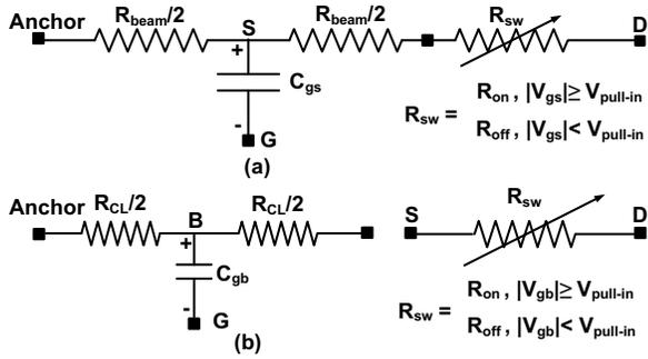
Figure 7. Electrical model of NEMS switch: (a) 3-terminal switch model; (b) 4-terminal switch model.
