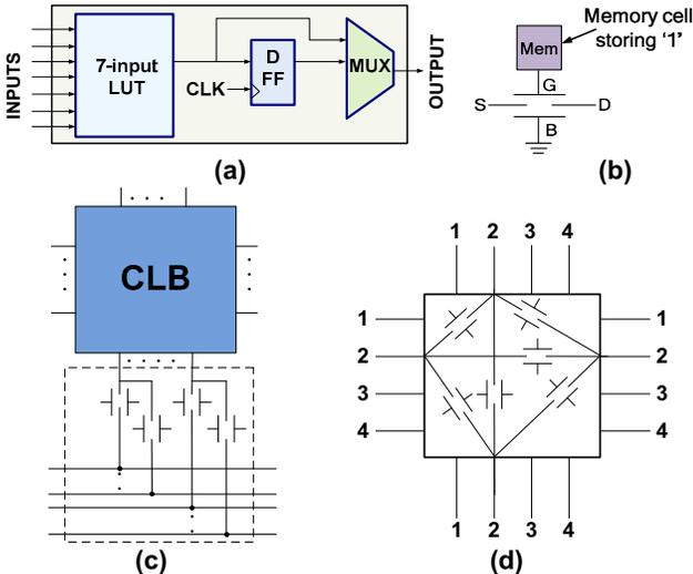
Figure 3. FPGA building blocks: (a) Configurable Logic Block (CLB); (b) PI routing switch; (c) Connection Box (CB); and (d) Switch Box (SB).
