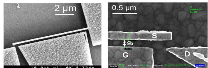
Figure 1. SEM picture of our fabricated laterally-actuated 3-T SiC NEMS switch (left); zoomed version to show the gap ( $g_0$ ) between the cantilever (S) and gate (G)/drain (D) electrodes (right).
