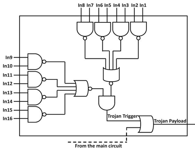
Fig. 7 An example comparator Trojan
