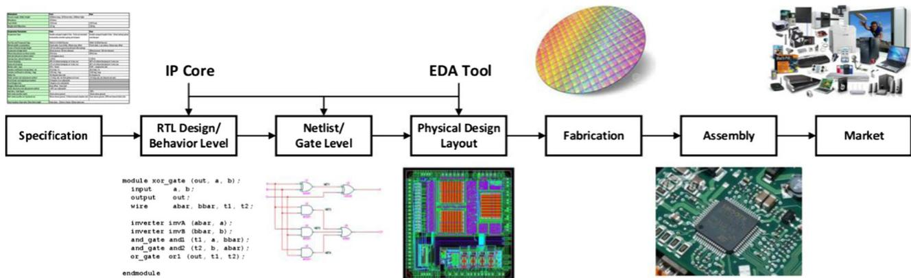
Fig. 1 Supply chain for IC production
