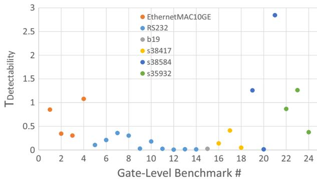
**Fig. 8** Detectability metric for gate-level Trojans in trust benchmarks
